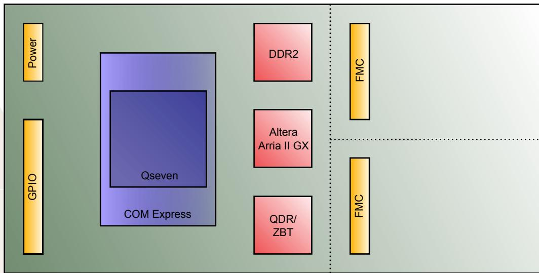
The carrier board with a connector for a COM Express or a Qseven CPU module and two FMC connectors for I/O modules. An Arria II GX FPGA, together with DDR2 and QDR/ZBT memories, is also shown.
